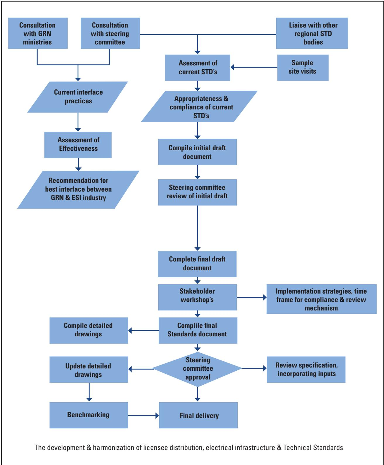
Figure 8: Distribution Electrical Infrastructure Project Flowchart
