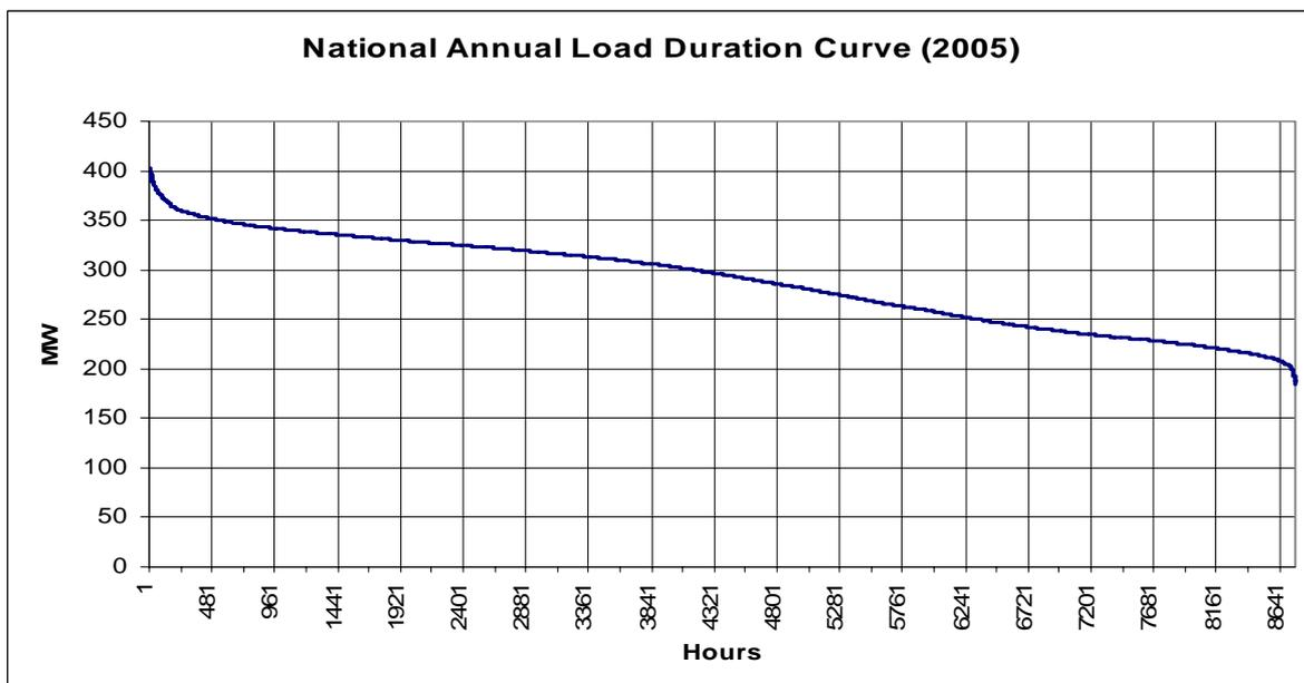
The figure above depicts the annual hourly load duration curve for the Namibian interconnected system for 2005. It is clear that there is a peaking requirement of at least 50MW and a base load requirement of between 200MW and 300MW. While Ruacana is a
