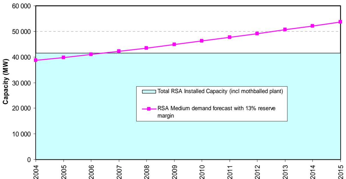
The above figure shows a RSA demand forecast vs existing capacity (source: NamPower). In 2006/2007 demand will overtake supply (or encroach on reserve margin). Significant amounts of new generation capacity have to be constructed to supply the forecast demand, and this does represent opportunities also for Namibian IPPs to sell into that market.
