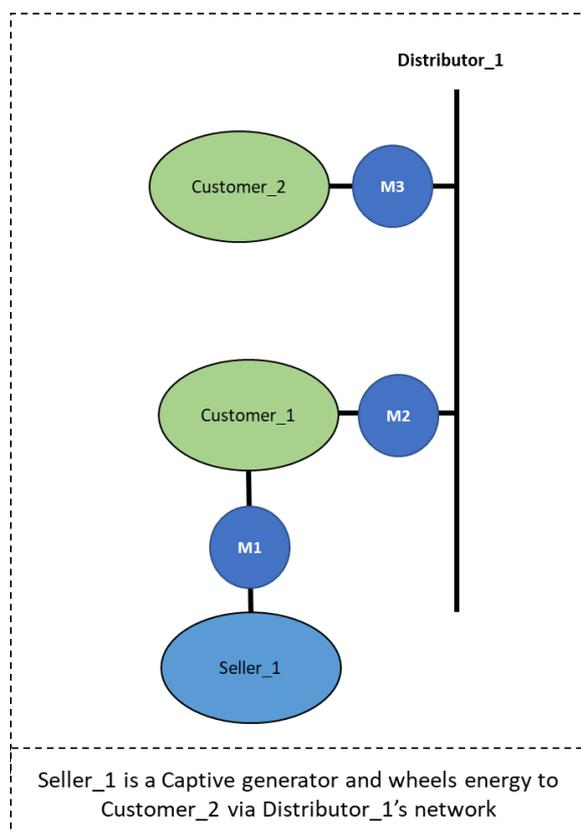
An add back could also be required in the event that a Distribution connected generator, wheels through the transmission network to another Distribution network. See figure below.
